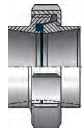
Complete ISO union S 2103 with Perbun sealing
